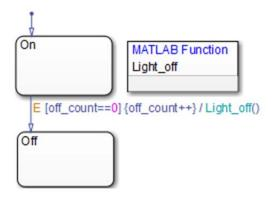
**Event Trigger**. Specifies an event that causes the transition to be taken, provided the condition, if specified, is true. Specifying an event is optional. The absence of an event indicates that the transition is taken upon the occurrence of any event. Specify multiple events using the OR logical operator (|).
