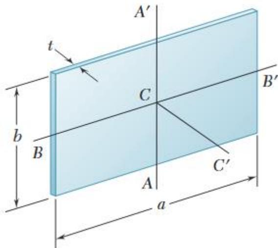
$$I_{AA'}, \text{ masa} = \rho t I_{AA'}, \text{ área} = \rho t \left( \frac{1}{12} a^3 b \right)$$
