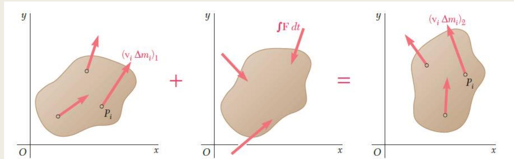
$$\text{Sist. Cant. Mov.}_1 + \text{Sist. Imp. Ext.}_{1 \rightarrow 2} = \text{Sist. Cant. Mov.}_2$$
