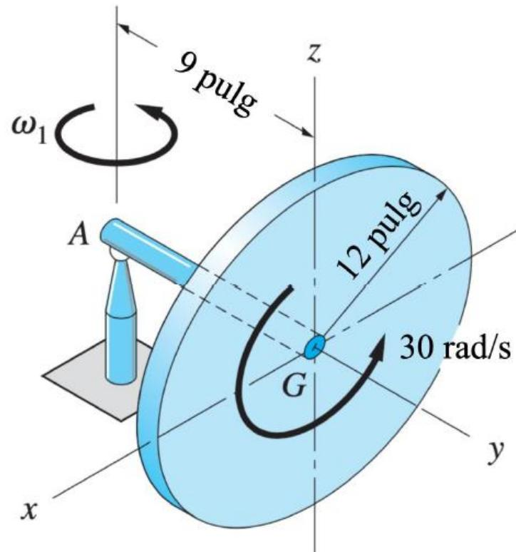
**Datos:** $m_{DISCO} = 25 \text{ lb}$     $\omega_{DISCO(AG)} = 30 \text{ rad/s}$  $\omega_{1 \text{ EJE } z} = \omega_1$ **Incógnita:** $\omega_1 = ?$  Eje permanezca horizontal
