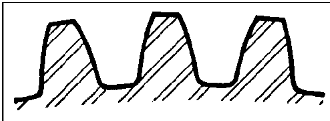
Paso diametral 2-1/2 - Paso Circular 1.2566"
