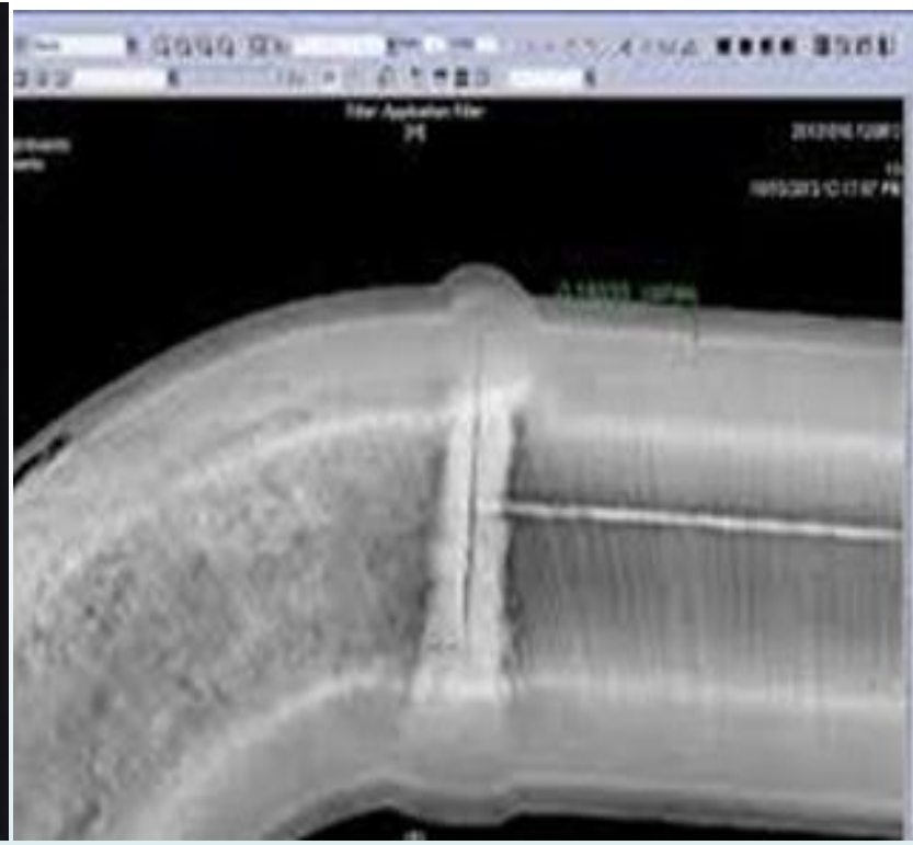
Transverse crack Feathery, twisting lines of darker density running across the width of the vessel image.
