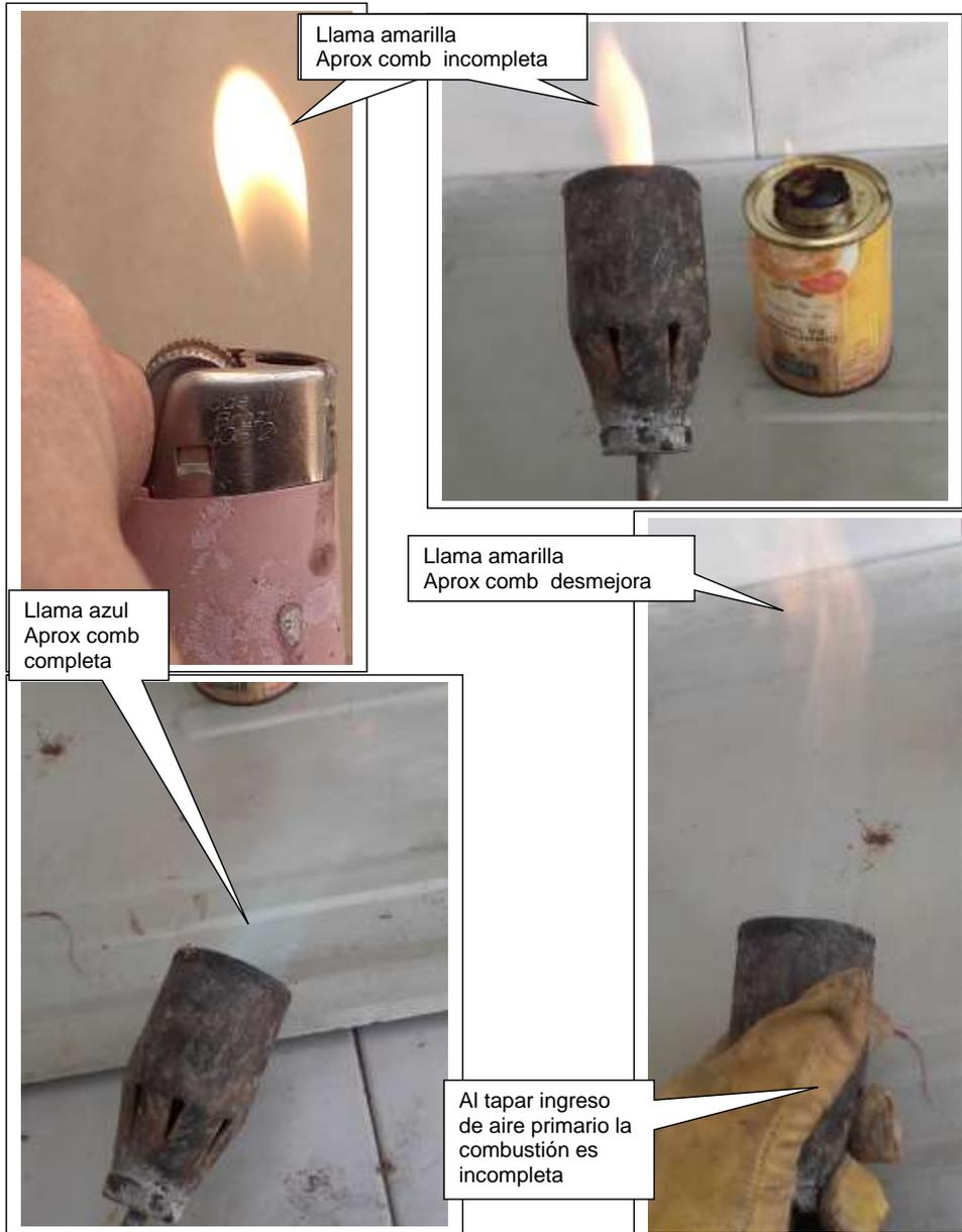
Fig Combustion Completa - Incompleta
