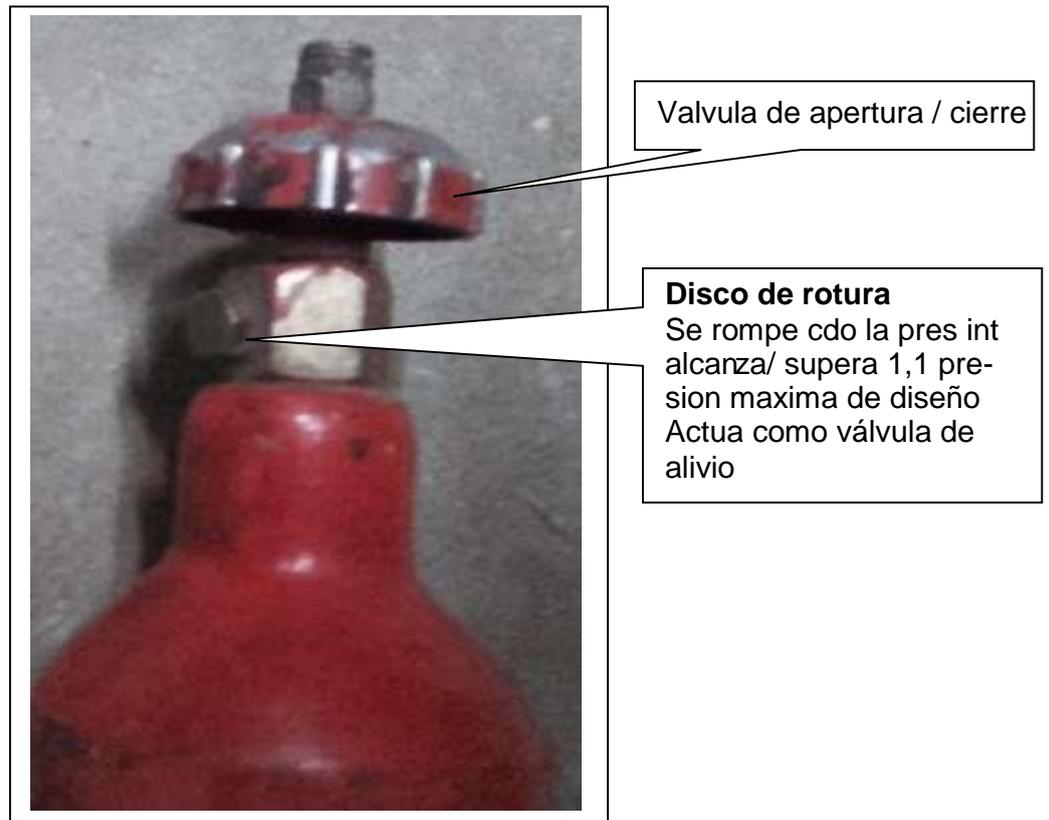
**Fig Ejercicio 4 Recip CO2 (extinguidor)**
