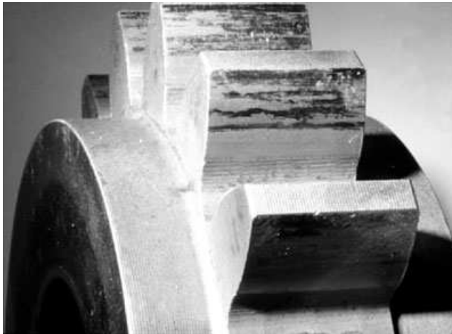
Fig. 10.13 Toothed wheel flank damaged by Micro-Pitting (PT-C-type, Micro-Pitting Test).
