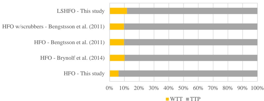
Figure 20: WTT and TTP relative contribution for GWP, in kg CO<sub>2</sub>e per tkm
