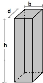
$$\gamma \left[ \frac{kg}{m^3} \right] \cdot b[m] \cdot d[m] \cdot h[m] = \text{peso propio columna}$$
