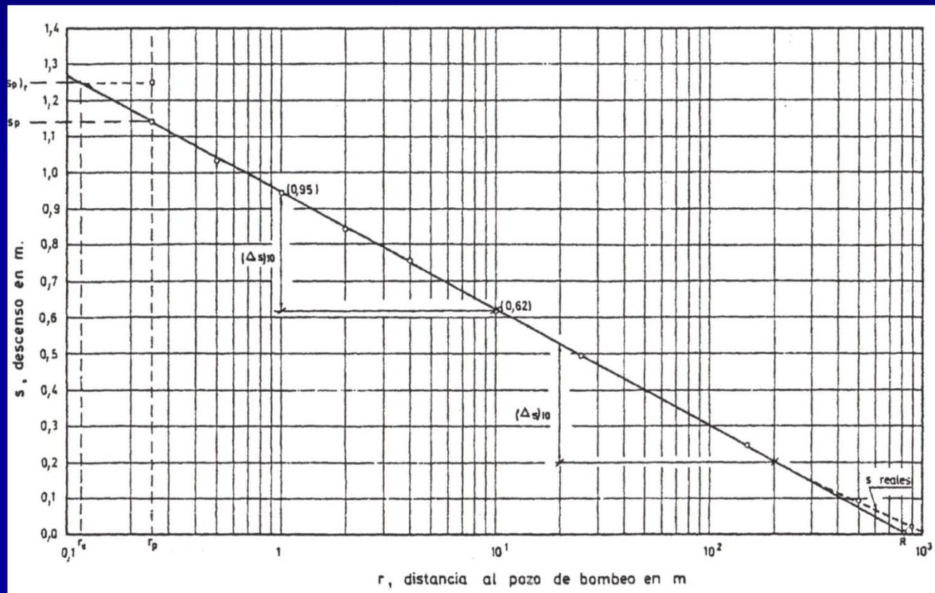
$$s_1 - s_2 = 2.3 \frac{Q}{2\pi T} \log \frac{r_2}{r_1}$$
