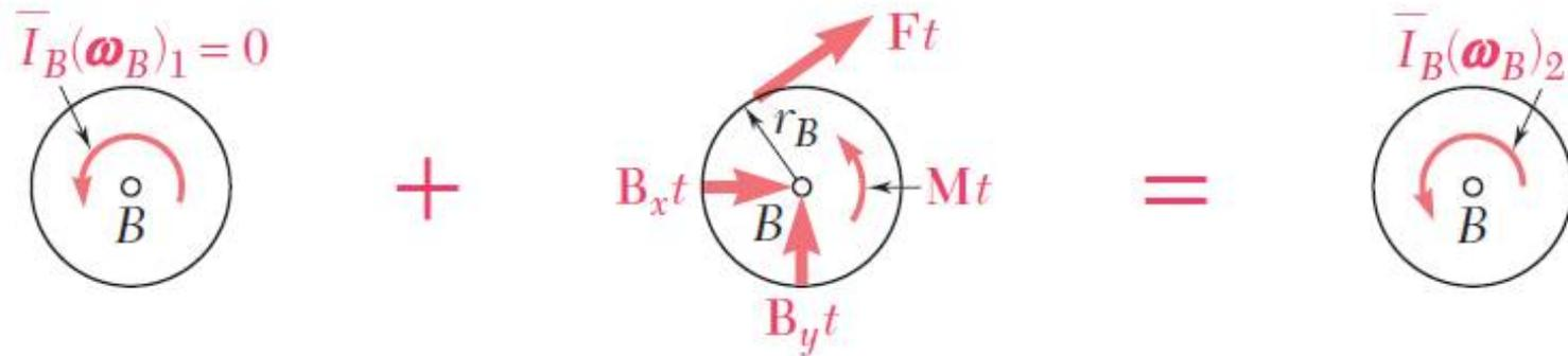
**Cant. Mov. Sist.<sub>1</sub> + Imp. Ext. Sist.<sub>1→2</sub> = Cant. Mov. Sist.<sub>2</sub>**
