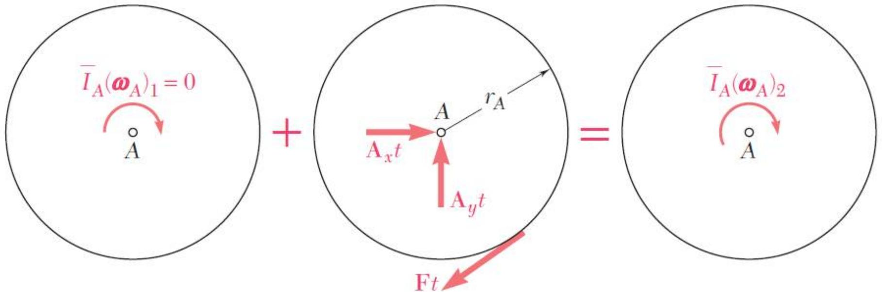
**Cant. Mov. Sist.<sub>1</sub> + Imp. Ext. Sist.<sub>1→2</sub> = Cant. Mov. Sist.<sub>2</sub>**
