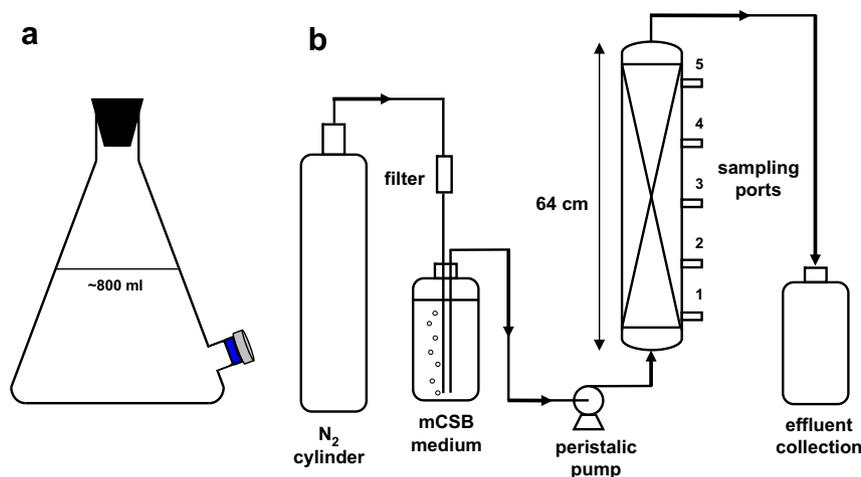
Fig. 2. Experimental set up for (a) batch culture and (b) up-flow packed-bed bioreactor experiments.
