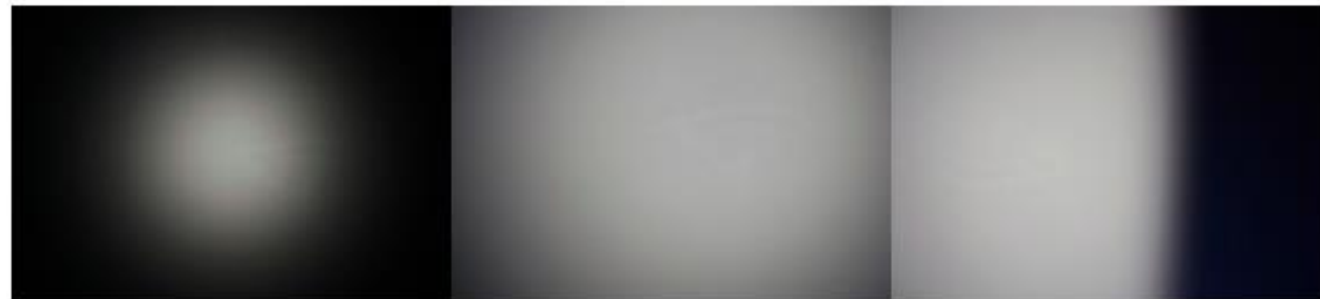
Light Field in Spot (left), Light Field in Flood (center), Barndoor Cut (right)
