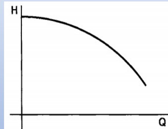
Figure 2.5: Single line pump performance curve
