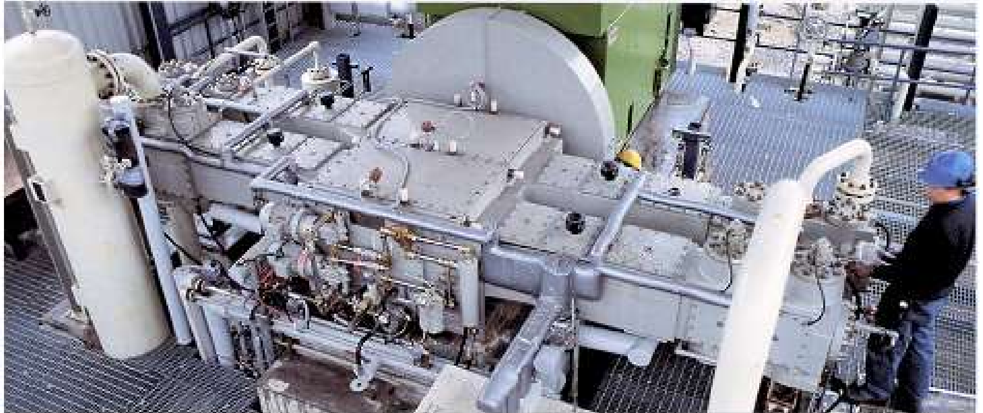
Figure 1-1. Typical horizontal balanced, opposed reciprocating compressor. (Source: Sulzer-Burckhardt, Winterthur, Switzerland.)
