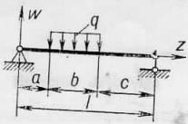
$$w(z) = -\frac{qbl^3}{48EJ} \left[ 8 \frac{d}{l} \left( \frac{z}{l} - \frac{z^3}{l^3} \right) - \frac{z}{l} \left( 8 \frac{d^3}{l^3} - \frac{2ab^2}{l^3} - \frac{b^3}{l^3} + 2 \frac{b^2}{l^2} \right) \right]$$
