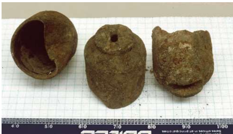
Fig. 4.6—Charge cases removed from a low-order gun.
