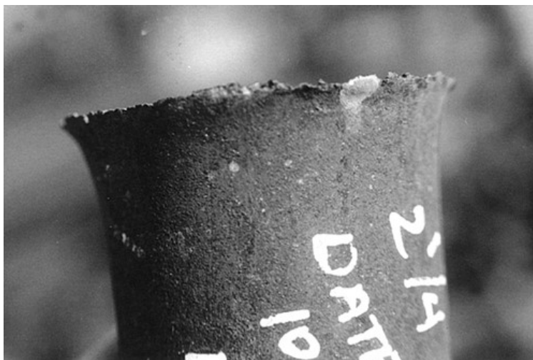
Fig. 4.13—Flare produced after explosive cutoff.
