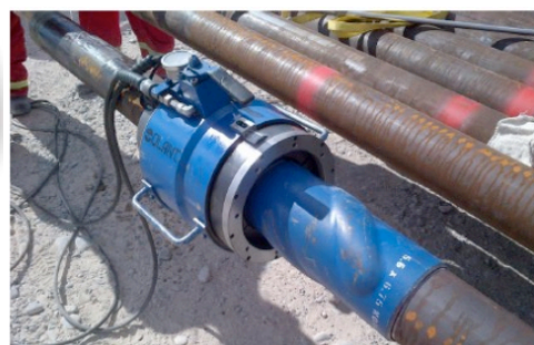
Tesco's patented RTF™ (Radial Tubular Forming) crimping technique
