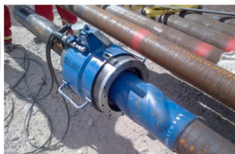
Tesco's patented RTF™ (Radial Tubular Forming) crimping technique
