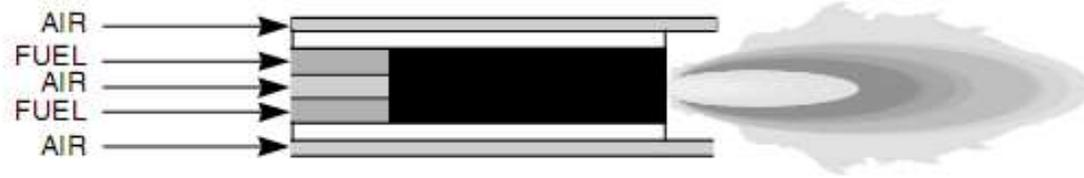
FIGURE 1.25 Schematic of a partially premixed burner.<sup>29</sup>
