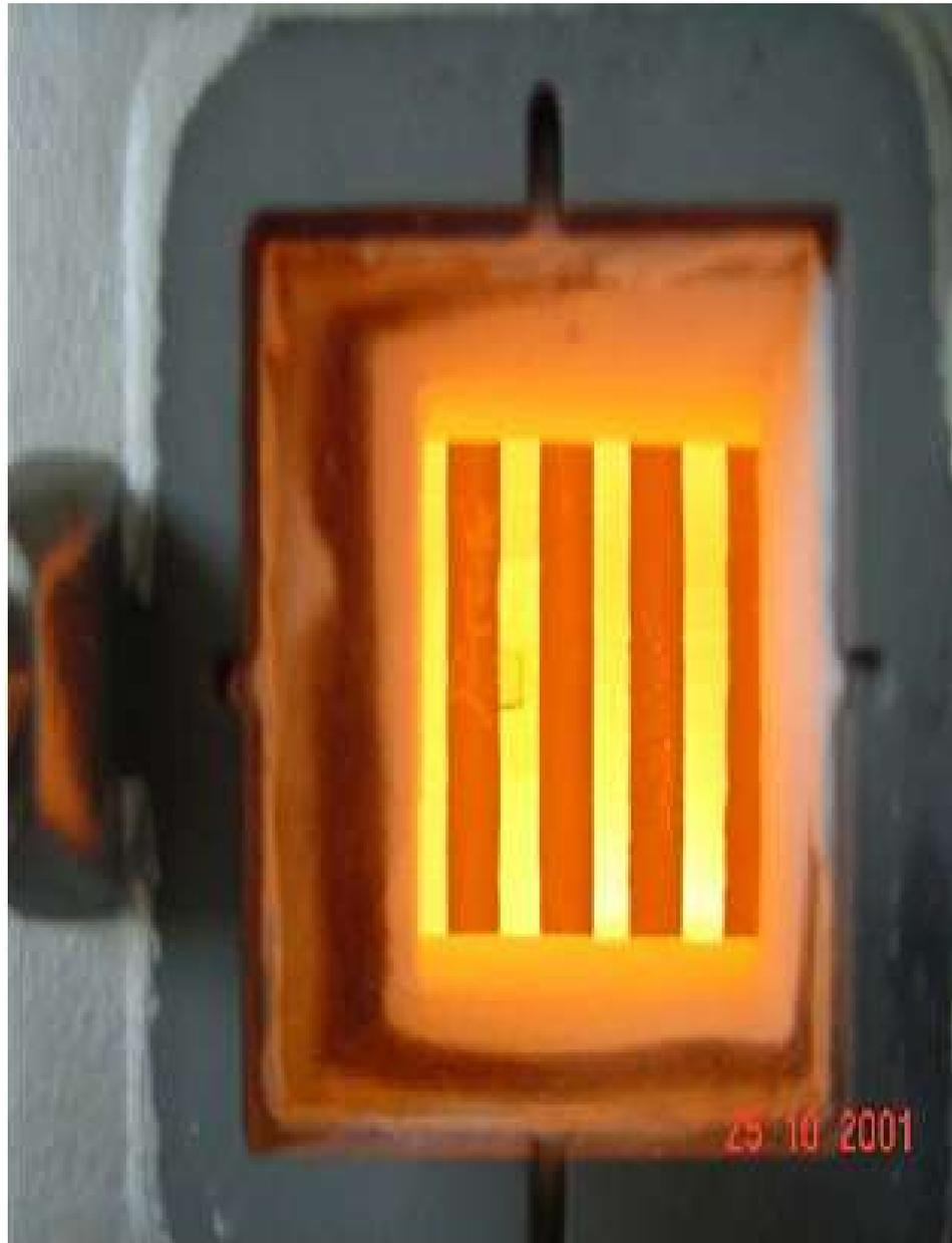
Radiant Coils in Normal Operation
