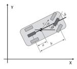
Vehicle data:  $v_0 = 12 \, m/s$ a = 2 m $b = 4 \, m$
