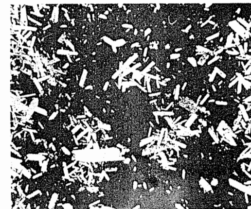
Fig. 10.13. Large grains of \text{Al}_2\text{O}_3 growing by secondary recrystallization from a fine-grained matrix. Courtesy I. B. Cutler, in reference 5.
