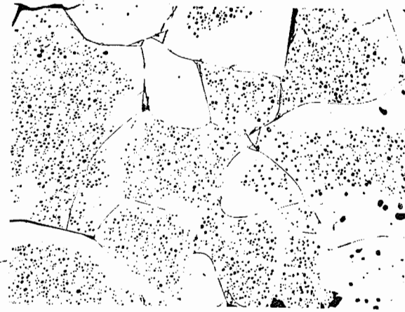
Fig. 10.33. Sintered \text{Al}_2\text{O}_3 , illustrating elimination of porosity adjacent to grain boundaries with residual porosity remaining at grain centers. Courtesy J. E. Burke.
