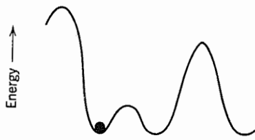
Fig. 18.10. Potential wells in a glass structure.
