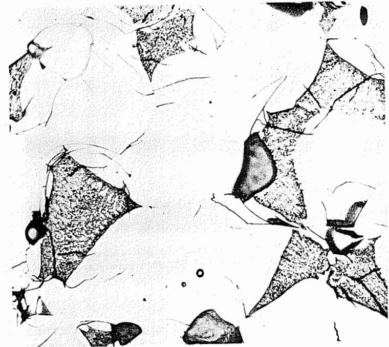
Fig. 11.32. Microstructure of two-phase ferrite ceramic. Light phase is \text{MgFe}_2\text{O}_4 , dark phase (\text{MgFe})\text{O} . Cracks due to microstresses are evident (500 \times ). Courtesy R. E. Carter.
