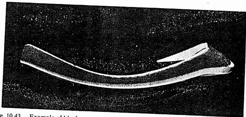
Fig. 10.43. Example of black core produced when time allowed for oxidation reactions was insufficient for completion of the reaction.
