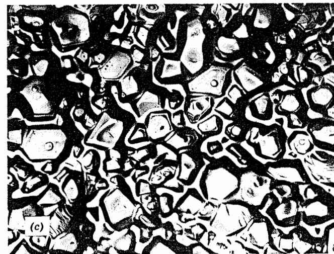
Fig. 10.40. (a) Surface of solid-liquid composite with varying amounts of liquid phase. (b) Drop of liquid between two solid spheres exerts pressure to pull them together. (c) Surface of forsterite ceramic showing liquid capillary depression between crystals.
