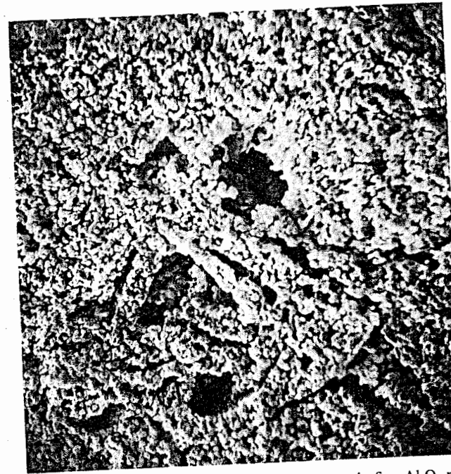
Fig. 10.32. Large voids formed by bridging of agglomerates in fine Al_2O_3 powder viewed with scanning electron microscope at 2000 \times . Courtesy C. Greskovich.
