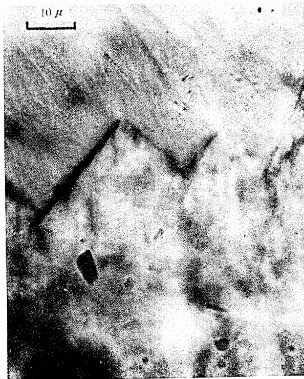
Fig. 8.8. (a) Interface morphology of \text{Na}_2\text{O} \cdot \text{SiO}_2 . From G. S. Meiling and D. R. Uhlmann, Phys. Chem. Glasses , 8, 62 (1967).
