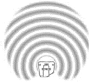
Forward-beaming radiation ~ 120 degrees 400 Hz – 2.5 kHz
