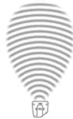
Narrow forward radiation ~ 40 degrees 2.5 – 10 kHz
