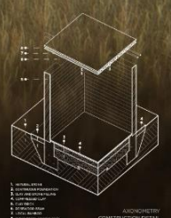
AXONOMETRY CONSTRUCTION DETAIL
