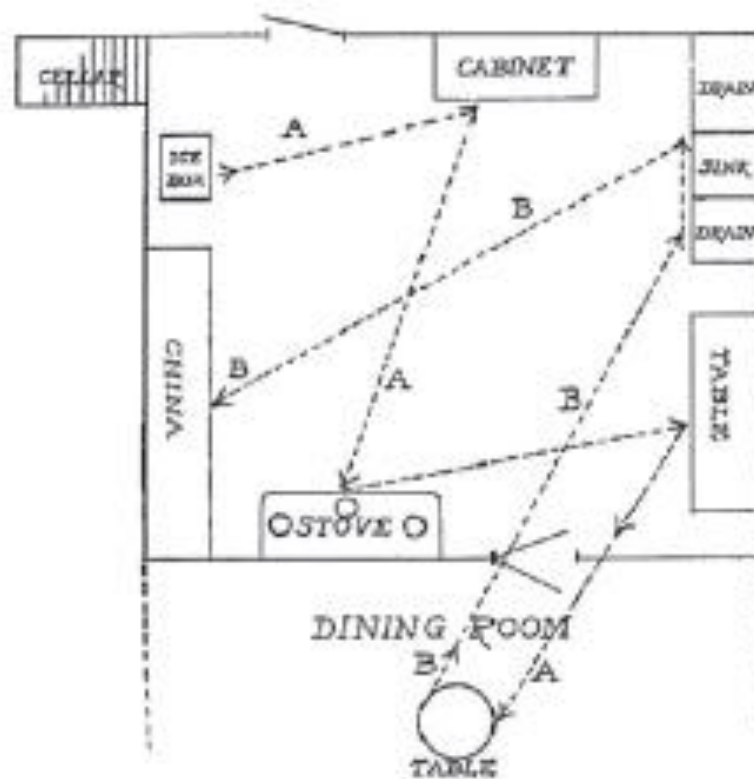
Diagram showing badly arranged equipment, which makes confused intersecting chains of steps, in either preparing or clearing away a meal. (A — preparing; B — clearing)
