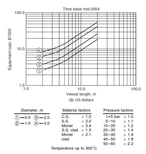
Figure 6.6a, b. Horizontal pressure vessels. Time base mid-2004. Purchase cost = (bare cost from figure)  $\times$  Material factor  $\times$  Pressure factor
