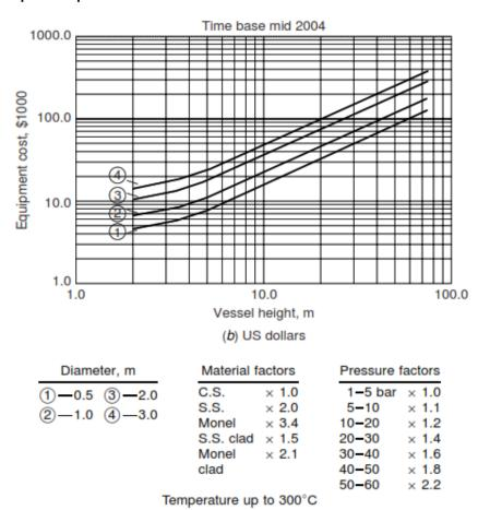
Figure 6.5a, b. Vertical pressure vessels. Time base mid-2004. Purchased cost = (bare cost from figure)  $\times$  Material factor  $\times$  Pressure factor
