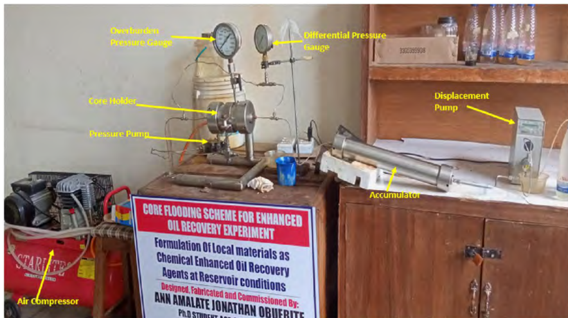
Figure 2—Core flooding experimental setup
