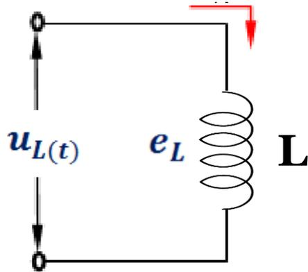
$$u_L(t) = -e_L = +L \frac{d(I_{max} \text{sen} \omega t)}{dt}$$
