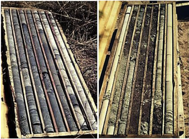
Fig. 20. Core of sandstone, siltstone and mudstone immediately after recovery (left) and after several months of storage in a core shed (right).
