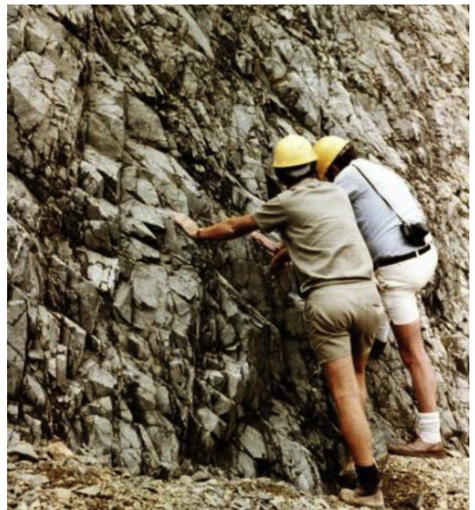
Fig. 1. Interlocking blocks of very strong Panguna andesite and granodiorite in the Bougainville open pit mine in Papua New Guinea for which the original Hoek–Brown criterion for rock mass strength estimation was developed (Hoek and Brown, 1980a, b).
