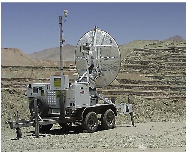
Fig. 27. Radar equipment for monitoring slope displacements.
