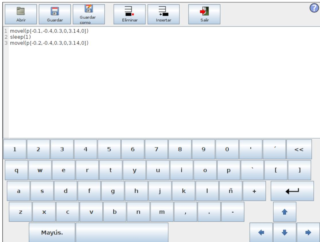
The screenshot shows the URScript editor interface. At the top, there is a file menu with the following options: "Abrir" (Open), "Guardar" (Save), "Guardar como" (Save as), "Eliminar" (Delete), "Insertar" (Insert), and "Salir" (Exit). Below the menu is a text area containing three lines of code:
