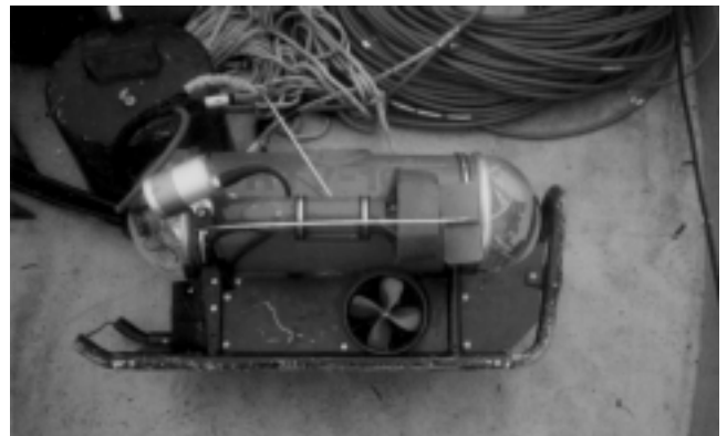
Fig. 1.4—Remotely operated vehicle (ROV). (Courtesy of M. Garlich.)
