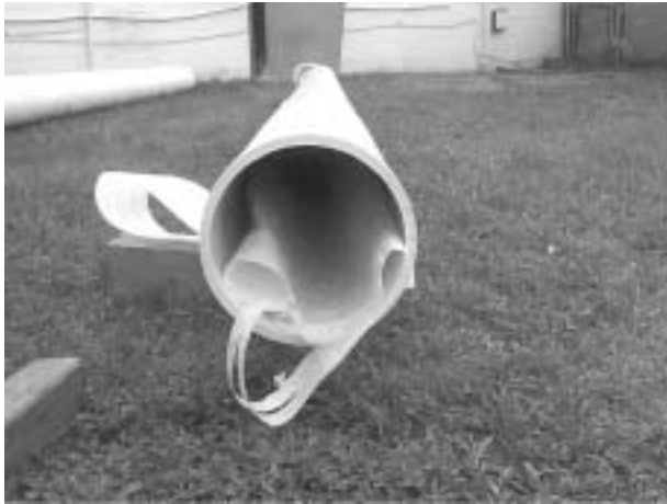
Fig. 5.13—Thin reinforced cementitious pole.
