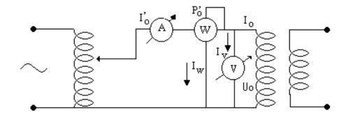
$$\begin{split} I_{0} &= I_{0}^{'} - I_{W} - I_{V} = I_{0}^{'} - \frac{U_{0}}{R_{W}} - \frac{U_{0}}{R_{V}} \\ P_{0} &= P_{0}^{'} - P_{W} - P_{V} = P_{0}^{'} - \frac{U_{0}^{2}}{R_{W}} - \frac{U_{0}^{2}}{R_{V}} \end{split}$$
