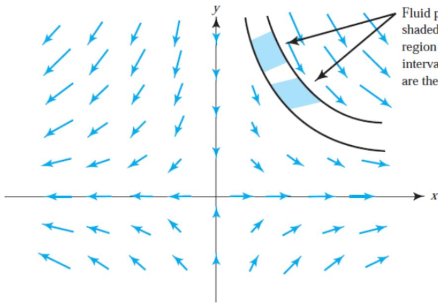
Fluid particles move from shaded region to shaded region after a fixed time interval. The two areas are the same.
