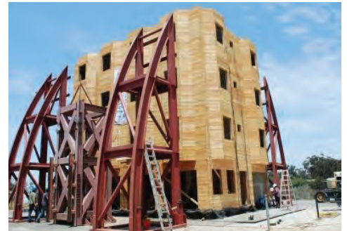
Earthquake simulations on the world's largest outdoor shake table at the University of California, San Diego, test retrofits to help buildings withstand earthquakes.
