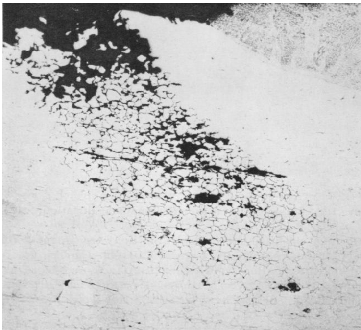
Fig 13. Weld decay (original magnification, \times 50 ).
