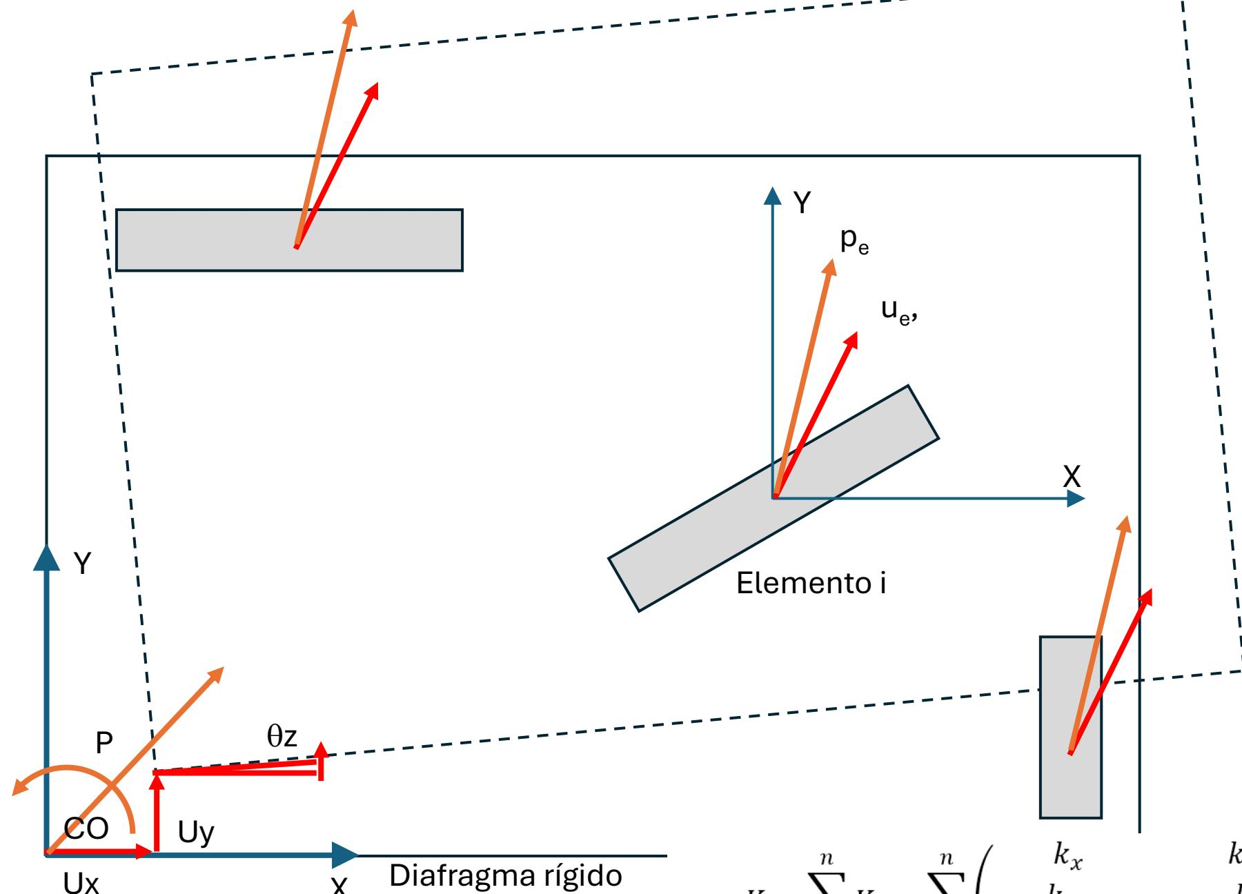
$$K = \sum_1^n K_e = \sum_1^n \begin{pmatrix} k_x & k_{xy} & k_{xy}x - k_xy \\ k_{xy} & k_y & k_yx - k_{xy}y \\ k_{xy}x - k_xy & k_yx - k_{xy}y & k_xy^2 + k_yx^2 - 2k_{xy}xy \end{pmatrix}$$
