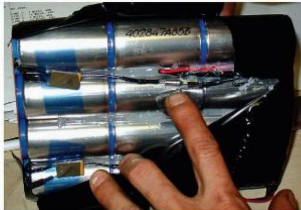
**Figure 17.** Photograph of a 9-volt AMF Battery Pack.
