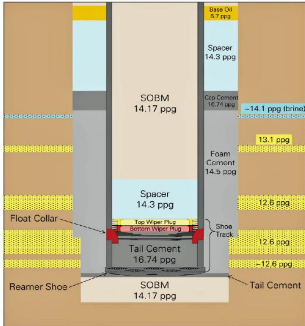
Figure 2. Planned Cement Slurry Placement.
