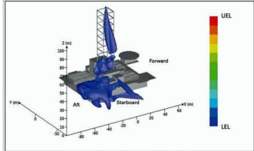
Figure 22. Vapor Dispersion Aft Deck—190 Seconds.
