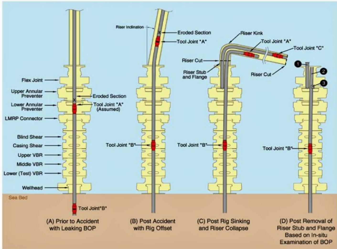
**Figure 15.** A Schematic of Drill Pipe Configuration Across the BOP Over Time.
