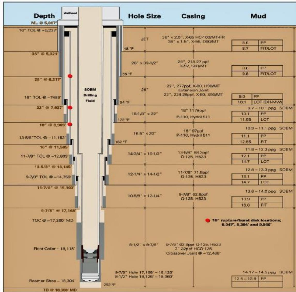
Figure 3. Actual Casing Run.
