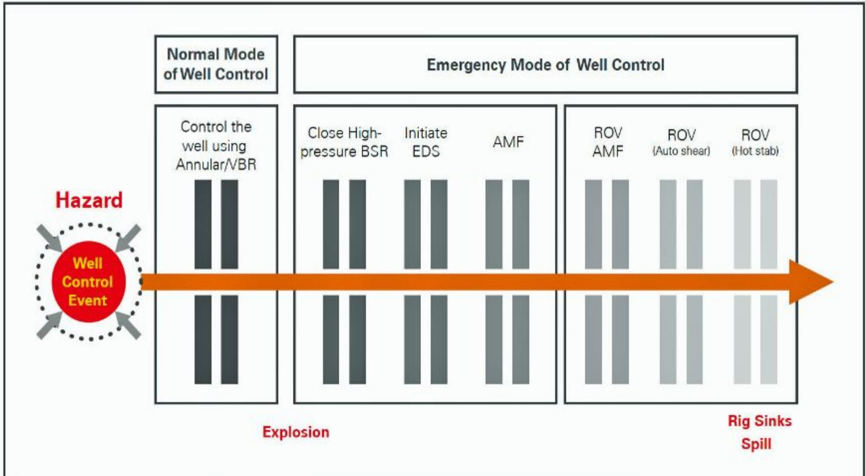
Figure 20. BOP Well Control Modes of Operation.
