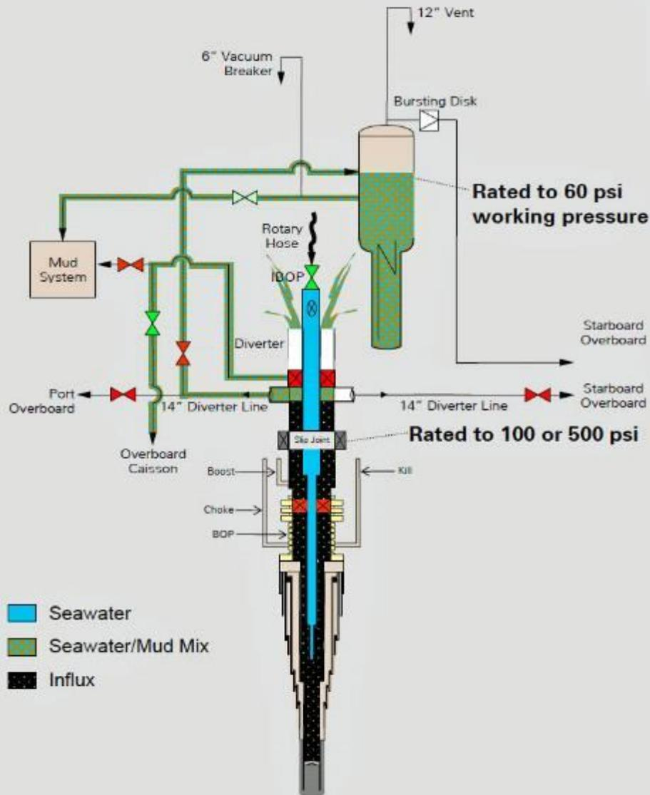
*When responding to a well control event the riser diverter is closed and fluids sent to either the mud gas separator or to the overboard diverter lines.*
