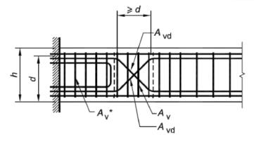
For sliding shear in downwards direction
