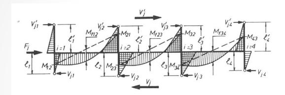
$$\begin{aligned} V_{j}^{'}+F_{j}+V_{j}&=\sum_{i}V_{ji}^{'}+F_{j}+\sum_{i}V_{ji}=0\\ \sum_{i}M_{ci}+\sum_{i}\Delta M_{i}^{'}&=\sum_{i}M_{ci}=cons\tan te \end{aligned}$$
