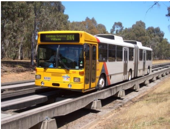
Fig. 7. Autobus. O-Bahn guide-way, Adelaida, Australia Fig. 8. Autobus guide-way. Alemania
