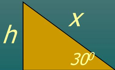
$$\text{sen } 30^\circ = \frac{h}{x} \quad x = \frac{20 \text{ m}}{\text{sen } 30^\circ} = 40 \text{ m}$$
