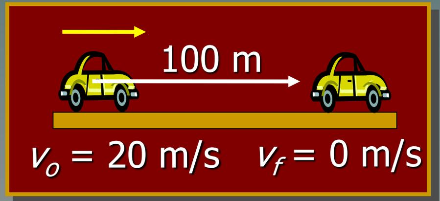
$$a = \frac{0 - v_0^2}{2s} = \frac{-(20 \text{ m/s})^2}{2(100 \text{ m})}$$
