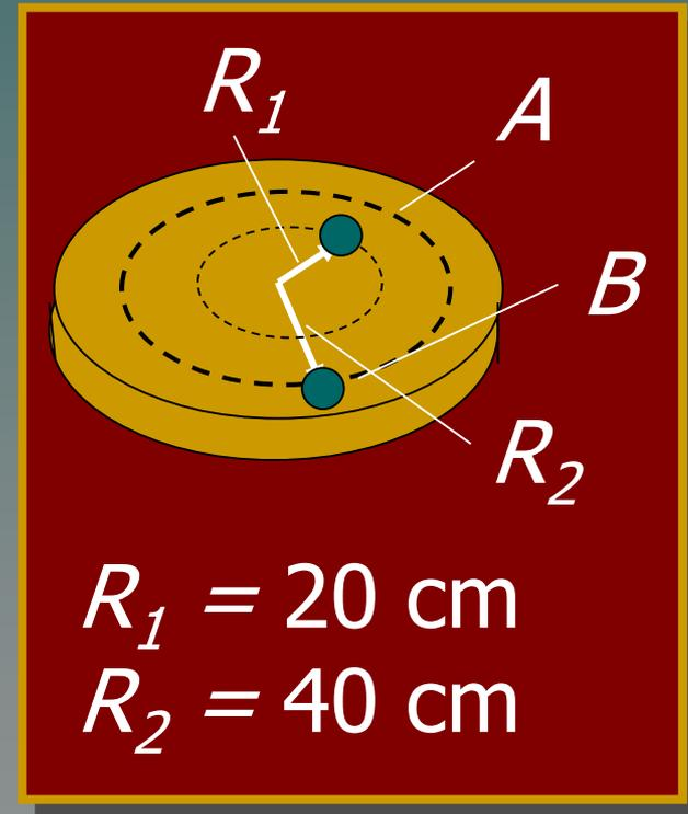
$$v_{Af} = \omega_{Af} R_1 = (20 \text{ rad/s})(0.2 \text{ m}); \quad v_{Af} = 4 \text{ m/s}$$
