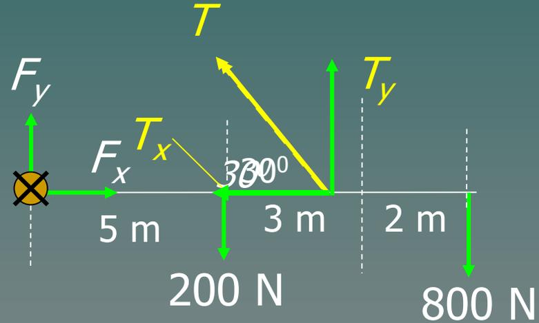
$$\Sigma F(\text{arriba}) = \Sigma F(\text{abajo}): \quad T_y + F_y = 200 \text{ N} + 800 \text{ N}$$
