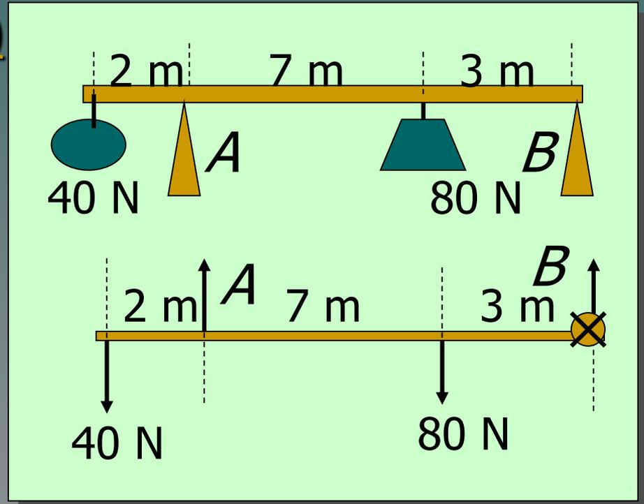
$$(40 \text{ N})(12 \text{ m}) + (80 \text{ N})(3 \text{ m}) = A (10 \text{ m})$$
