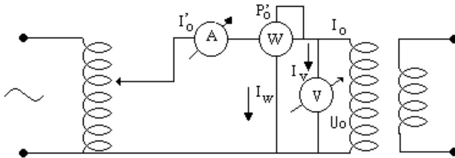
$$I_0 = I_0' - I_W - I_V = I_0' - \frac{U_0}{R_W} - \frac{U_0}{R_V}$$
