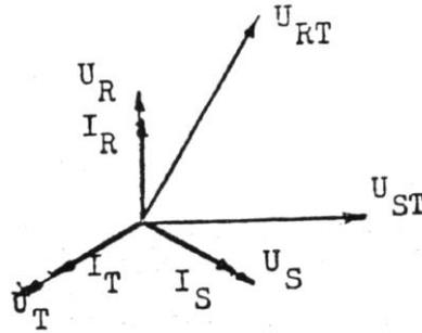
b- Carga  $Z_R = Z_S = Z_T = R + j X$ ;  $\frac{X}{R} = \text{arctg} 30^\circ$
