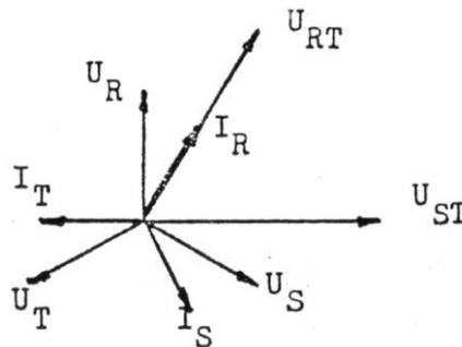
c- Carga  $Z_R = Z_S = Z_T = R + j X$ ;  $\frac{X}{R} = \text{arctg} 60^\circ$
