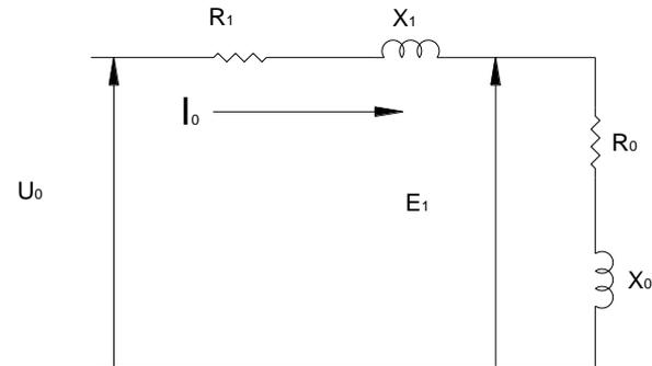
Para determinar  $X_0 \Rightarrow \frac{U_1}{I_0} = Z_{eq} = \sqrt{(R_1 + R_0)^2 + (X_1 + X_0)^2}$
