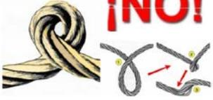
CABLE DOBLADO POR DESENCOLLADO INCORRECTO Y POSTERIOR ESFUERZO
