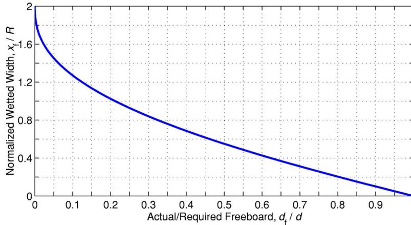
**Figure 3.** Normalized wetted width of tank roof,  $x_f/R$  as a function of actual/required freeboard,  $d_f/d$ .
