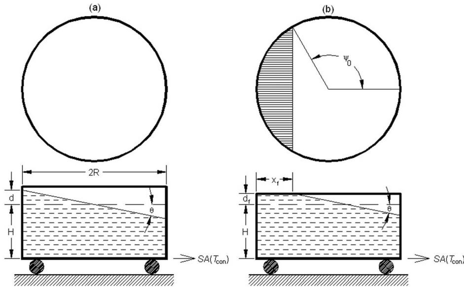
**Figure 2.** Liquid-filled tank translating with an acceleration  $SA(T_{con})$ : (a) sufficient freeboard, and (b) insufficient freeboard.
