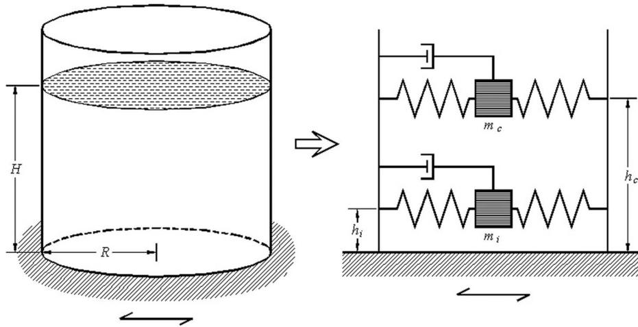
Figure 1. Simple model of liquid-filled tank.
