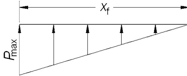
**Figure 4.** Radial variation of pressure on tank roof.
